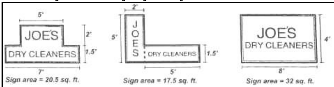
Figure 1 Sign Measurement Area
